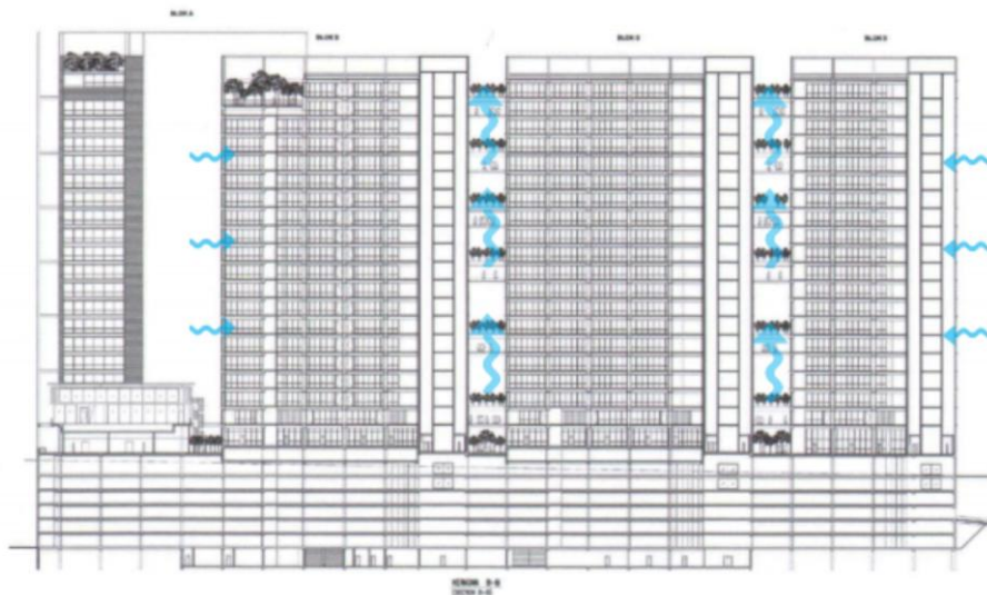
Figure 5.1: Stack ventilation effect at PJ Trade Centre
